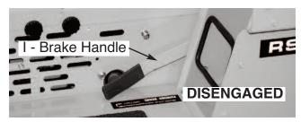
and behind "inside face" of Carriage Bolt. To "disengage" Parking Brake, reverse the above procedure and allow Brake Handle to rest on Fender.
