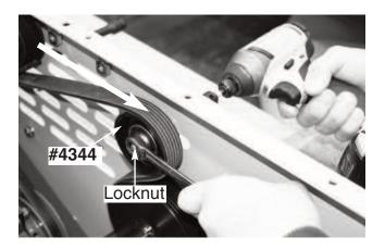
**9.** Add proper tension to the #4356 Micro-V belt by inserting a 3/8" drive socket ratchet in the square hole in the #4341 auto tensioner. While pushing towards the rear of the tractor, carefully slide the #1521 Tension Bar out of the body of the RS1000, being careful of engine wires, etc. (See picture at the top of the next column).
