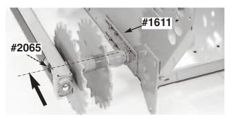
**3.** With gloved hands, begin to rotate the Track forward. [TIP: As you rotate the Track, you may want to move the Track Clutch Controls back and forth to relieve any "drag" from the Track Clutch Belts].
