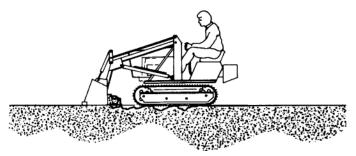
CAUTION: Exercise care when undercutting high banks. Soil slides can be dangerous. Load from the banks as low as possible for maximum efficiency. Remember that loader lift and break-away capacities diminish rapidly as loading height is increased.
