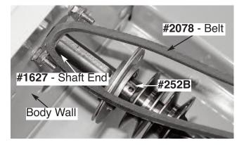
Lower Power Shafts! Shafts were factory aligned when the Crawler was manufactured to allow easy remounting of the Bearings that you have temporarily removed to create a "slot" on each Shaft end.
