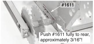
Using a "flat-nosed" punch and hammer, push the #1611 Front Axle Plate (located on both sides of Body) rearward till it hits a solid stop. **NOTE:** in the work done in steps above, this Plate may have already worked its way rearward. To check, push Plate forward from the rear, then push it back the required 3/16" distance.
