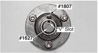
...make sure it's end hits the "V" slot "dead center". (Use this procedure for  ${\color{black}{both}}$  the Upper &
