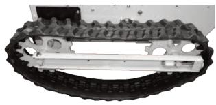
**3.** With gloved hands, begin to rotate the Track forward. [TIP: As you rotate the Track, you may want to move the Track Clutch Controls back and forth to relieve any "drag" from the Track Clutch Belts].
