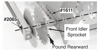
**3.** Slide #2065 Axle fully rearward. **HINT:** With a mallet, gently pound rearward on the front idler sprocket teeth. Do the same to the other side as well. Work back and forth until both left and right front idler sprockets are all the way rearward. The #1611 Front Axle Plate should have moved to its' most rearward position.
