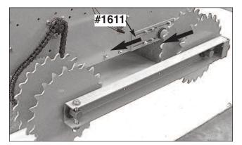
**1.** Remove the remaining locknuts from the left and right tension bolts. Your front tension bolt assembly should be loose. At this time, remove all remaing bolt assembly parts and pull out #1810 Tension Bolt. Put items aside, in order, for later reassembly. **Do to both sides of tractor.**
