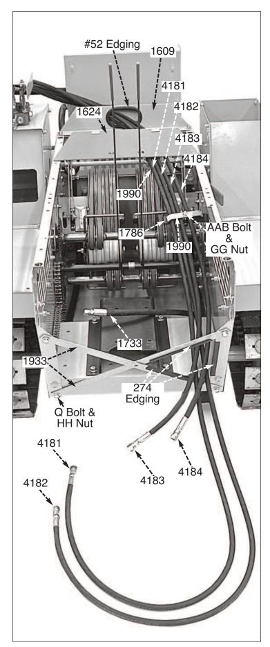
STEP 27. Loop remaining ends of Hoses #4181, #4182, #4183 and #4184 through the #52 Rubber Edged "hole" in rear outside center of #1609 Spanner. Continue forward going *fully under* #1624 Bridge and finally *over* #1786 Bracket... secure above Hoses with #1990 Clip and AAB Bolt & GG Nylon Nut... leave Nut loose.
