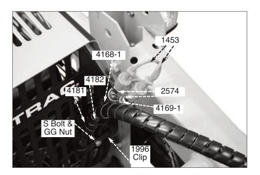
STEP 11. In order from left to right if standing in front of grill: Hoses #4181, #4182, #4168-1, #4169-1 should all be behind #1996 Clip held loosely by #SS Bolt & GG Nut.
