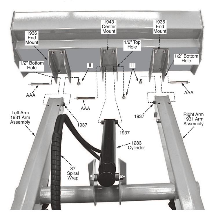
At this time, Fully Tighten all AH and X Spin Lock Bolts on your Bucket Assembly.
