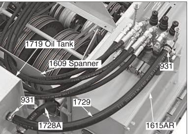
**STEP 15.** Screw #1738 Fitting into threaded port on right side of #1920 Valve Bank. Turn ... stop with tube of Fitting pointing directly rearward... tighten lock-nut on Fitting.
