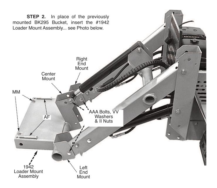
**STEP 2.** Align the #1942 Mount so that its Left, Right, and Center Mounts are in the identical position as the previous #1936 End Mounts and #1943 Center Mount were on the BK295 Bucket. Secure with the same #AAA Bolts, #VV Washers and #II Nuts used in the Bucket installation and tighten... check Photo above closely.
