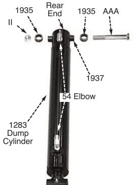
**STEP 50.** Insert #1937 Tube into "non-piston end" of #1283 Dump Cylinder per Photo at left. Over Left & Right ends of #1937 Tube slip on a #1935 Tube.
