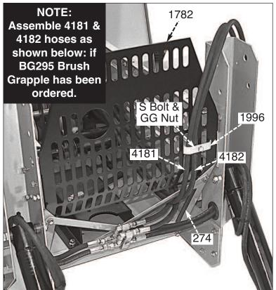
**STEP 10.** On the #1782 Grill, release the S Bolt & GG Nut so that #4181 & 4182 Hoses are loose... Photo at left.
