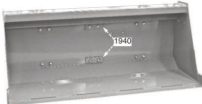
STEP 1. Insert four (4) AH Bolts into the four 3/8" holes on "inside face" of #1943 Center Mount. Apply this assembly to the pattern of four (4) 3/8" holes on center "rear face" of #1941 Bucket Assembly... insert Bolts into mating 3/8" holes.
