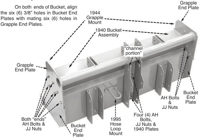
**STEP 3.** From outside, slip a #AH Bolt into each one of the six (6) mating holes aligned above on each end of Bucket. Inside Bucket secure Bolts with #JJ Nuts... finger tight. Using original four (4) AH Bolts, JJ Nuts and two #1940 Plates, mount "channel portion" of Grapple Tine Assembly into the same location you had previously removed #1943 Center Mount... finger tight.
