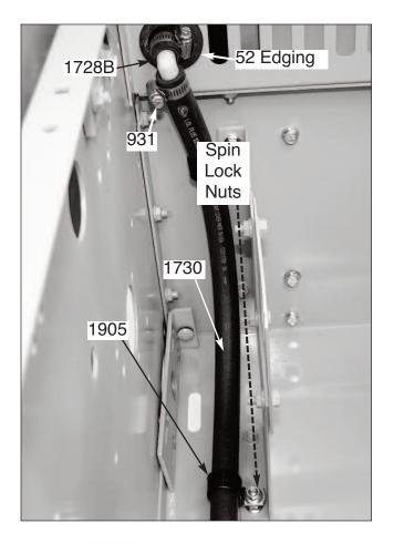
**STEP 3**. From "inside" Body slide remaining end of #1728B Hose through #52 Edging. Slip #1905 Coated Clip over remaining end of #1730 Hose... Photo at left.
