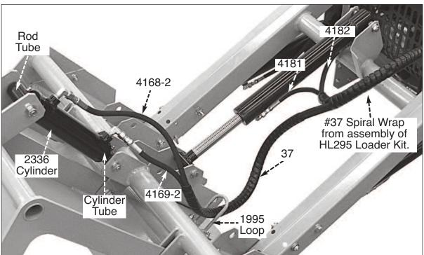
**STEP 15.** Follow Photo above and connect each of the Four (4) Hoses to their appropriate Cylinder Fittings... NOTE: Hoses #4168-2 & 4169-2 pass through bottom of #1995 Loop. Once happy with hose path...tighten hoses to fittings.
