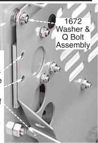
**STEP 40B.** Slip Q Bolt into two (2) #1672 Washers and from outside insert into 1" access hole of #1930R Right Upright and then into 5/16" hole in top front of Body Wall. Secure inside with HH Nut... tighten.
