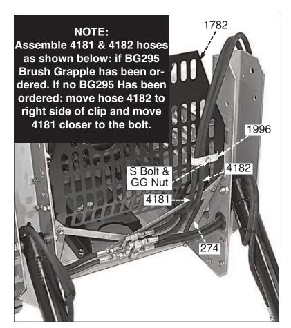
STEP 43. Replace your #1782 Front Grill if it was removed for previous assembly. Use R Bolts and HH Nuts to secure your assembly... tighten all six (6) Bolts and Nuts at this time... see Photo below.
