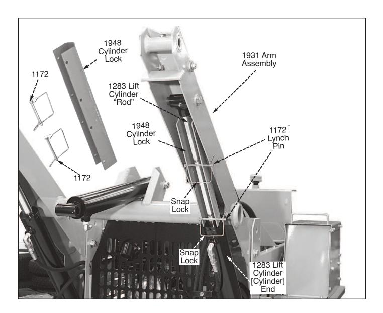
**STEP 58.** For Maintenance Safety, your Magnatrac RS1000 is equipped with a #1948 Cylinder Lock. This Lock must be in place when ever the Arm Assembly is raised and can not be supported on the ground.
