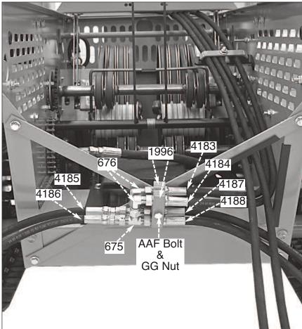
STEP 30. Attach a #676 Elbow to #4183 Hose. In a similar manner attach a #676 Elbow to #4184 Hose... only finger tighten both assemblies.
