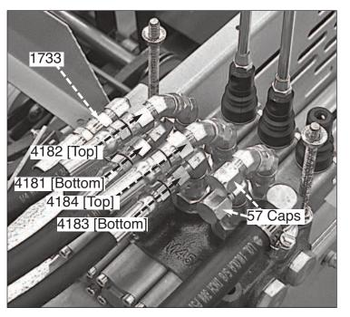
insert #1733 Hose through #1880 Grommet and connect with #1920 Valve.
