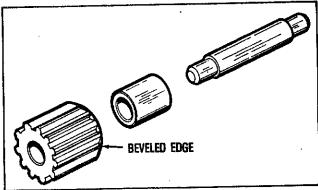
With the small gear of the three gear cluster toward the spacer, install the three gear cluster and other 1/32" thick by 7/8" I.D. thrust washer on the brake shaft.
