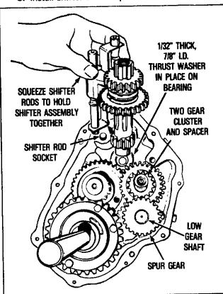
Install the reverse idler shaft, spacer and gear into the cover. The beveled side of the idler gear should be down into the cover.
