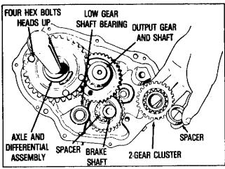
Remove the output shaft and gear and thrust washer from each end of the shaft.
