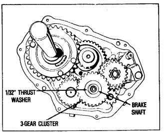
8. Remove the reverse idler gear, spacer and shaft from boss in cover.
