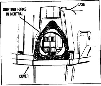
14. Align the case and cover with the two dowels, then install and tighten the eight socket head capscrews. Torque screws to 10 ft. lbs. Unit can now be placed flat on the work bench.
