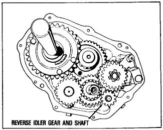
9. Lift out the shifter assembly. Service of this unit is described in Chapter 10.
