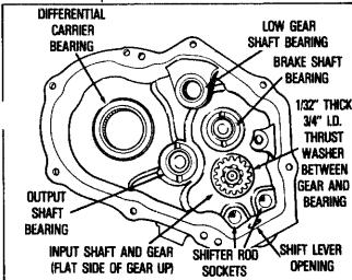
Center one 1/32" thick by 1" I.D. thrust washer on the cover brake shaft needle bearing, then install the brake shaft and gear, (chamfer side away from cover).
