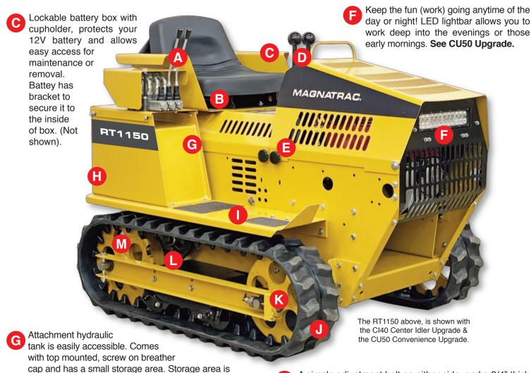
Hydraulic filter and drain are easily accessed on the back right of the hydraulic tank.
